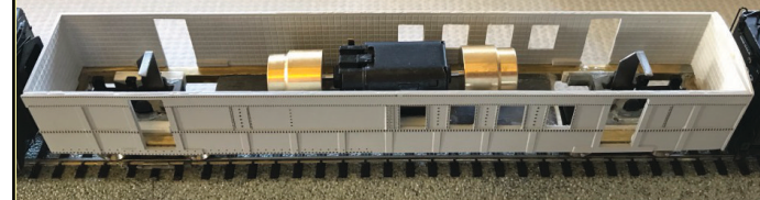
In-process scratch-built combine car. The modeler was attempting to model an entire eighteen-car NYC passenger train exactly. Problem - his Hudson can't pull an eighteen car train. Solution - install a drive train in the combine. Even RPMers sometimes make concessions!
