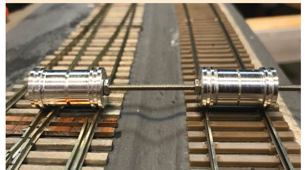
The relieved center of the rollers let it span diverging rails in a turnout. The threaded rod and lock nuts set track-to-track distance. Remove the rod from the rollers for flexibility
