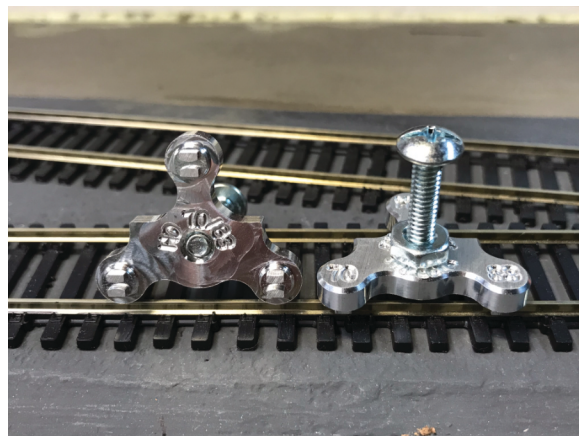
Trifectas are works of art. This photo shows the well-engineered rail lugs on the left (bottom view). Their interior is curved to accommodate curved track and milled to the NMRA flangeway clearance. They have a centerline indicator, removable handle, and engraved scale/code are also visible.
