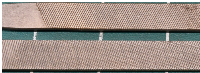
Photo 1. Single Cut top, Double Cut bottom. Both are No.2 Swiss Pattern
