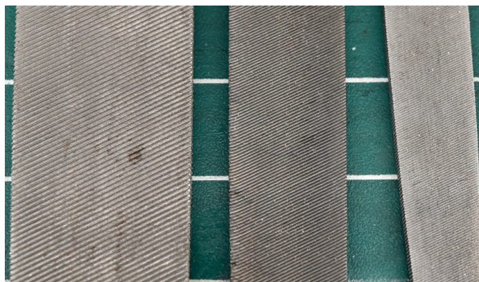
Photo 2. The 6" file in the middle and the 4" file on the right are both Smooth Cut, but have obvious tooth spacing differences. 10" Bastard Cut file on the left for reference
