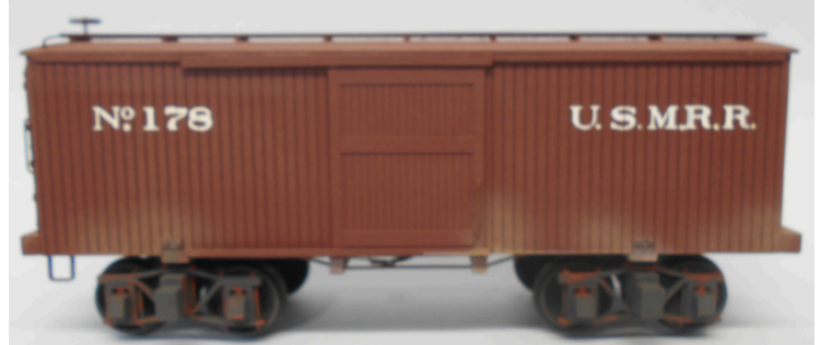
The Civil War-era USMRR boxcar was scratch-built in the 1980s. Jim also added a simple brake system to it.
