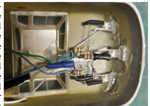
Figure 10 Multiple LEDs, resistors, and split light bar.
