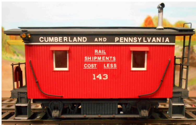
extensively modified with new styrene sides, among other things. The lettering used dry transfers and cobbled decals. The model was built in the late 1980s.
