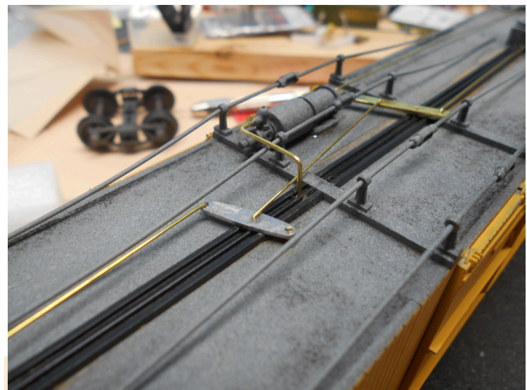
Interurban under-body updated brake system.
