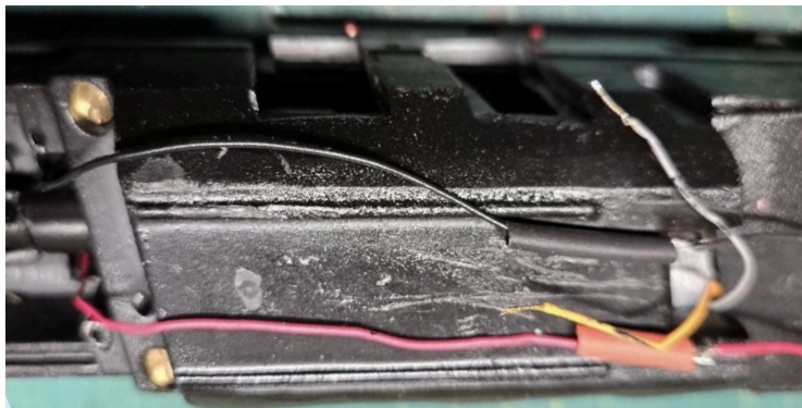
Figure 7 Underbody fitting into the frame and wiring.
