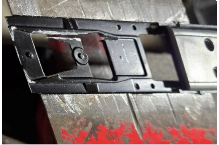
Figure 2 Upside down frame in a clamp after filing off burrs.
