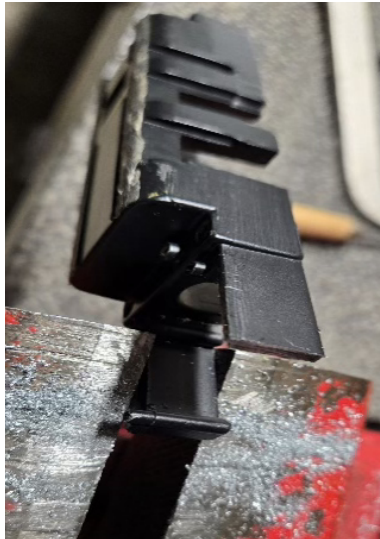
Figure 6 Frame in clamp for filing.
